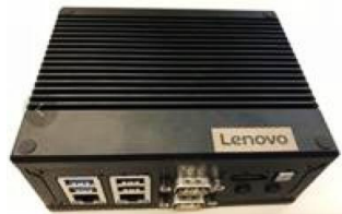
2x USB 3.0 Ports 2x USB 2.0 Ports Power Button
